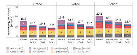
[Figure 5: Energy Use Intensity (kWh/sq. ft. per year) – (CZ4c) Mixed Marine]
