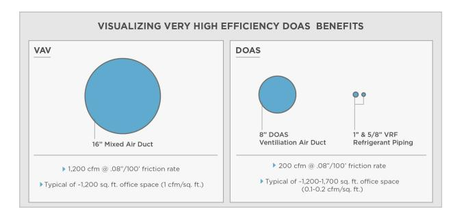
[Figure 3: Saving Space Through Duct Size Reduction]
