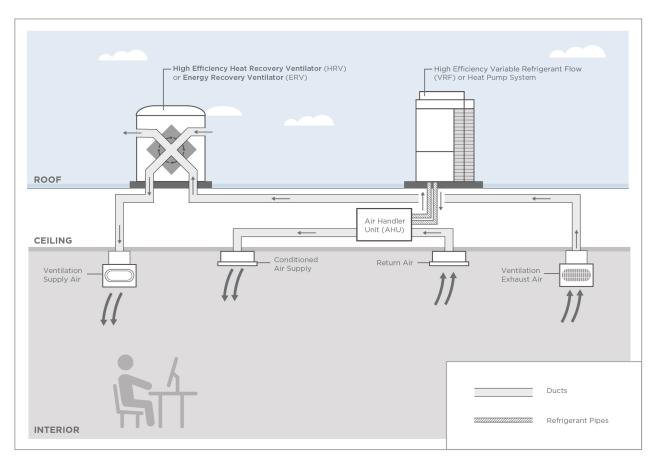
[Figure 2: Very High Efficiency DOAS Schematic]
