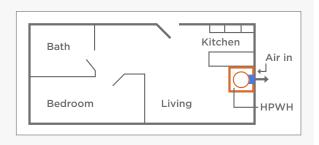
TS5: Split-system HPWH with tank in unit and outdoor unit placed on exterior.
